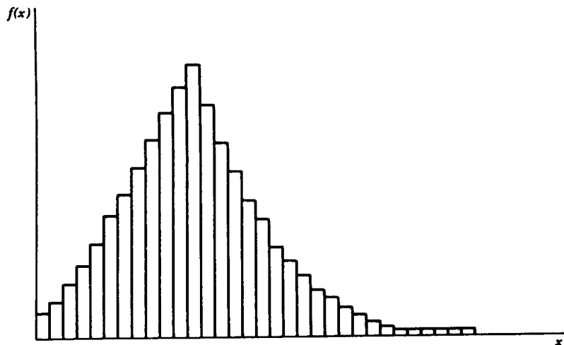
Figure 4.5.1 A histogram resulting from a large number of values and small class intervals.
